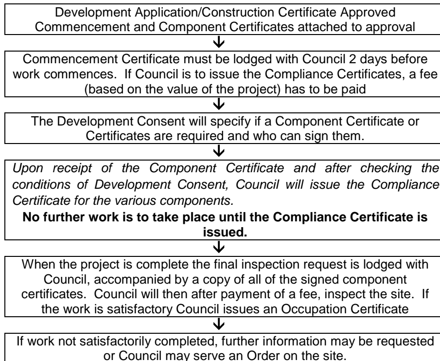
Fig 2 Post Development Application/Construction Certificate Flow Chart
